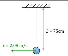
At the bottom of its swing, the ball is traveling 2.08 m/s when the string suddenly breaks.
