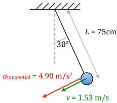
A mass is attached to the end of a 75.0-centimeter long light string which is then attached to the ceiling, and allowed to swing back and forth as a simple pendulum. When the pendulum makes an angle of  $30.0^{\circ}$  with the vertical, it has a tangential acceleration of  $4.90 \text{ m/s}^2$  and a tangential velocity of 1.53 m/s, as shown.
