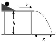
In a lab experiment, a ball is rolled down a ramp so that it leaves the edge of the table with a horizontal velocity v. If the table has a height h above the ground, how far away from the edge of the table, a distance x, does the ball land? You may neglect air friction in this problem.
