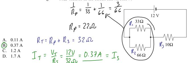
32. What is the total power dissipated by the three resistors in the circuit shown below?
