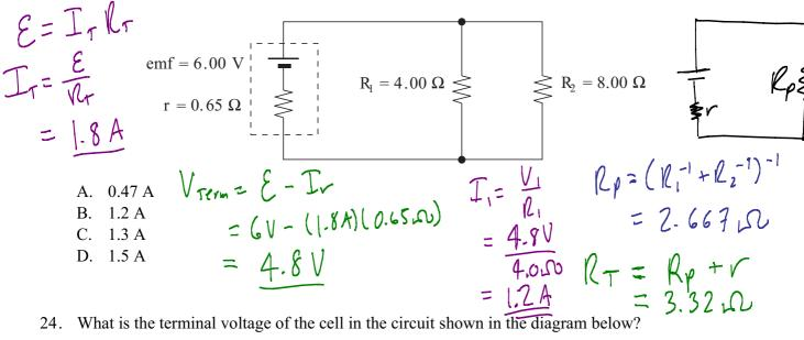
24. What is the terminal voltage of the cell in the circuit shown in the diagram below?
